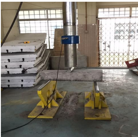
Figure 12. Determination of flexural strength
