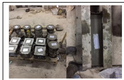
Figure 5. Casting of cubes, cylinder and beams
