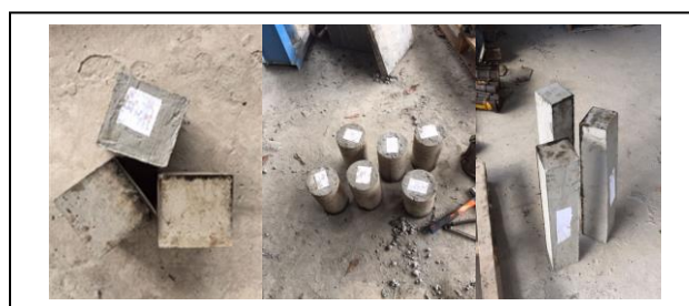
Figure 6. Specimen after removing molds
