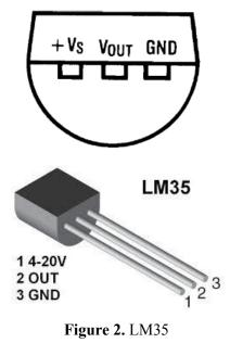
LM35 is a precision IC temperature sensor with its output proportional to the temperature (in oC). The sensor circuitry is sealed and therefore it is not subjected to oxidation and other processes. With LM35, temperature can be measured more accurately than with a thermistor. It also possess low self-heating and does not cause more than 0.1 oC temperature rise in still air.
