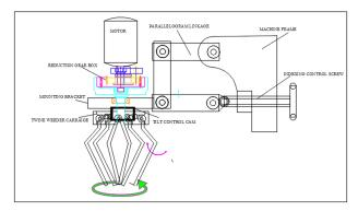
Figure 1. Design of the Kinematic linkage for weeder
