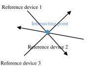
Figure 1 Concept of Triangulation by distance interception
