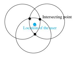
Figure 2. Concept of Triangulation using multiple interception points
