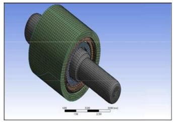
Figure 3. Mesh Generation of Whole Assembly
