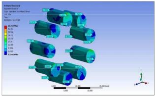
Figure 12. Equivalent Stresses for Rollers
