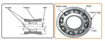
Figure 1. Rolling Bearing
