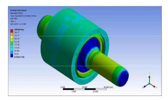
Figure 7. Equivalent Stress Plot
