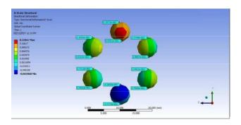
Figure 15. Directional Deformations for Balls (Y-axis)
