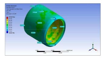
Figure 16. Equivalent Stresses for Sleeve
