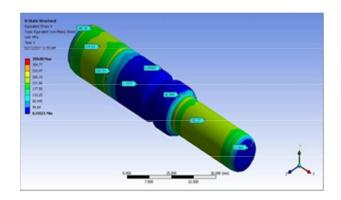
Figure 10. Equivalent Stresses for Shaft
