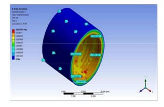
Figure 9. Total Deformation for housing
