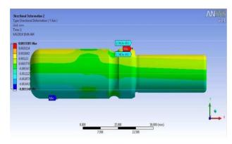
Figure 11. Deformations for Shaft (Y-Direction)
