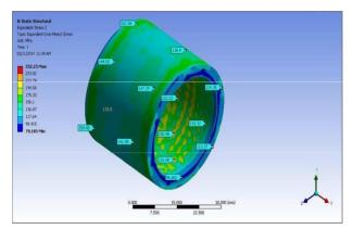
Figure 8. Equivalent Stress for housing
