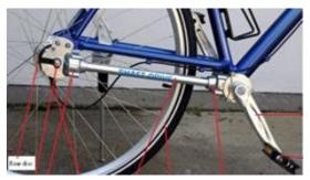
Figure 3. Components of shaft driven bicycle
