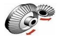
Figure 4. Bevel Gear
