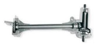
Figure 2. Shaft drive for bicycle
