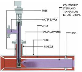
Figure 1: Venturi type de-superheater
