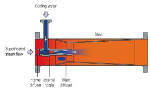
Figure 2: Working of venturi type de-superheater
