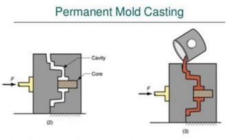
Steps in permanent mold casting: (2) cores (if used) are inserted and mold is closed, (3) molten metal is poured into the mold, where it solidifies.
