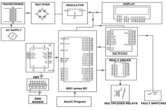
Figure 1. Block Diagram
