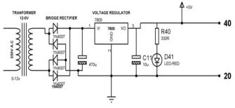
Figure 2. Power Supply Diagram
