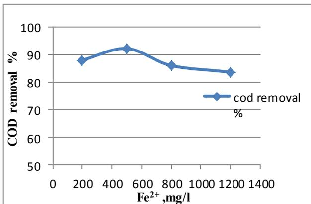
**Figure 2.** Effect of Fe<sup>2+</sup> concentration on COD removal
