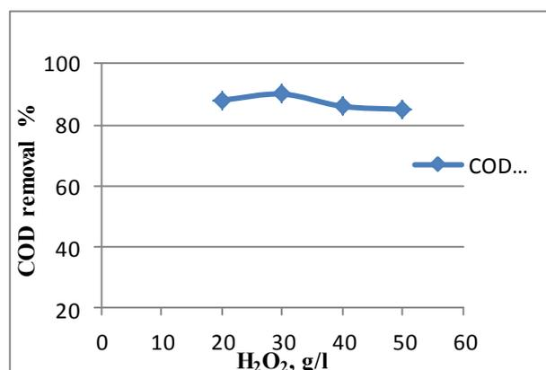
Figure 1. Effect of H<sub>2</sub>O<sub>2</sub> concentration on COD removal
