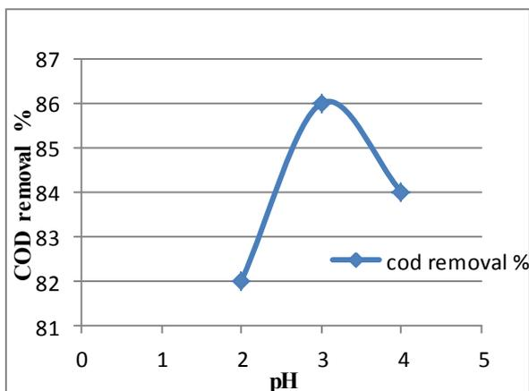
**Figure 3.** Effect of pH on COD removal
