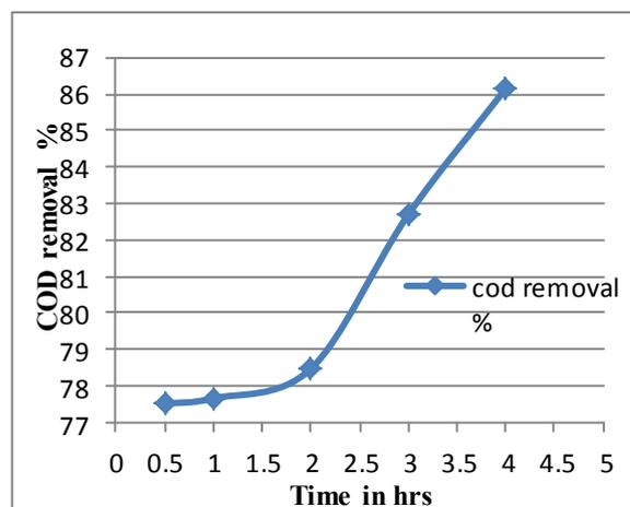
**Figure 4.** Effect of reaction time on COD removal
