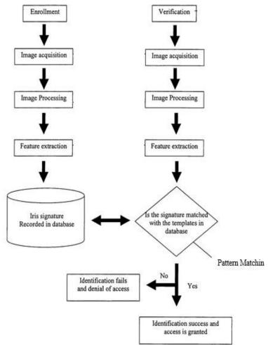
Figure 3. Block diagram of Iris recognition system
