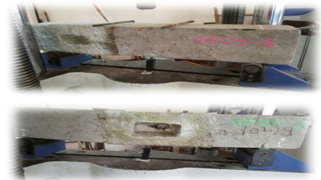
Fig 8: -Test setup for beams with opening wrapped using C.S.M
