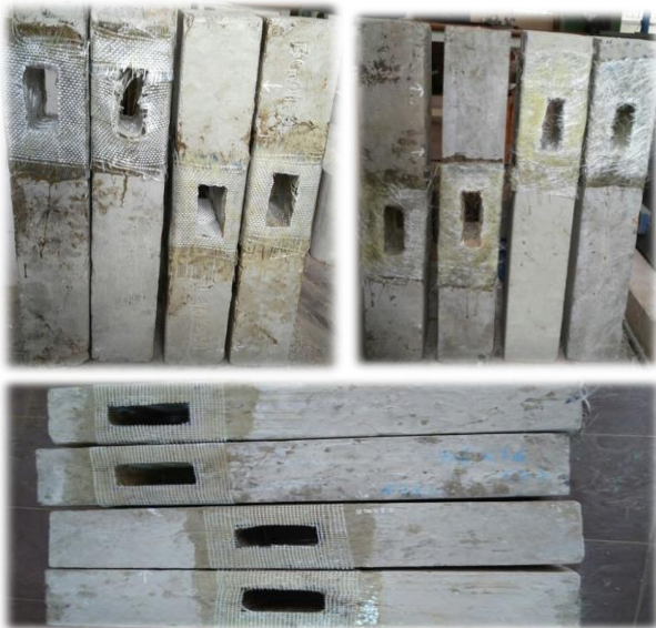
Fig 5: - opening wrapped using W.R, CSM and Mesh
