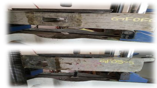
Fig 9: - Test setup for beams with opening wrapped using Mesh
