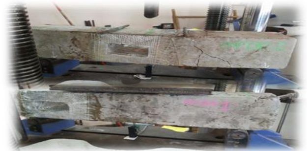
Fig 7: - Test setup for beams with opening wrapped using W.R
