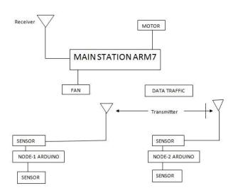
Figure1. Block diagram of main station ARM7
