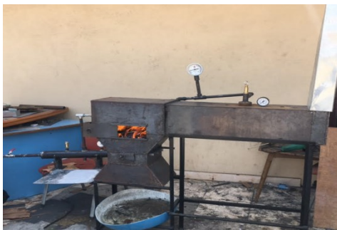
Figure 8 Final Designed Super Heater
