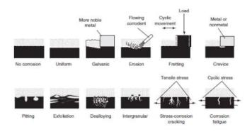
Figure 1. Different Forms of Corrosion
