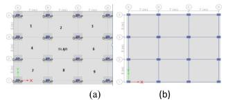
Figure 1: layout of model a) flat slab model b) conventional slab model
