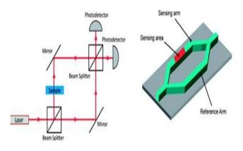
Figure 2: MZ modulator inner view
