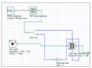
Figure 6: Subsytem-2 (Transmitter Section)
