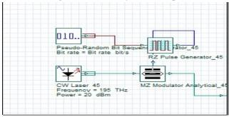
Figure 5: Subsystem-1(Transmitter Section)
