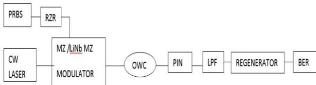
Figure 1 : Layout design of the inter-satellite communication system
