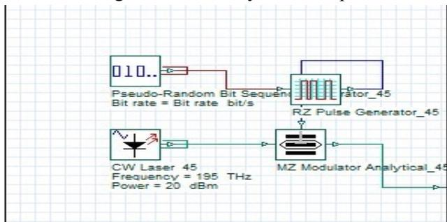
Figure 5: Subsystem-1(Transmitter Section)
