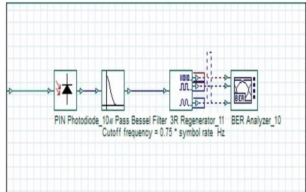
Figure 7: Subsystem-3 (Receiver Section)
