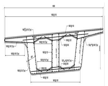
Figure 9: Reinforcement detailing of the section at anchorage
