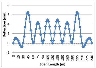
**Figure 7:** Deflection due to DL and PSG along the entire span of the bridge
