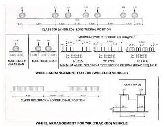
Figure 4: wheel arrangement for 70R wheeled and 70R tracked vehicle
