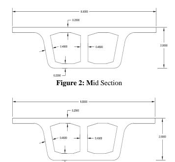
Figure 3: Section at column
