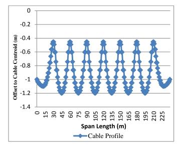
Figure 6: Tendon profile for the entire span of bridge
