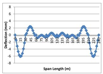
**Figure 8**: deflection due to DL, SIDL, LL and PSG along the entire span of the bridge
