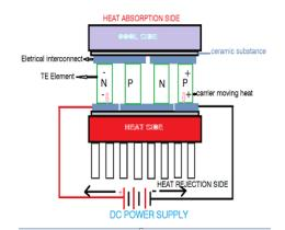
Figure 1. Thermo Electric Module
