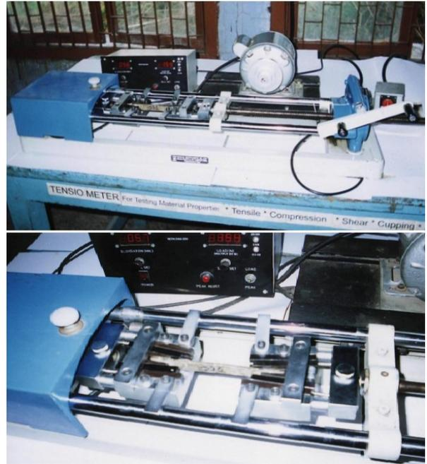
**Figure 6.** Strength measuring equipment Tensiometer
