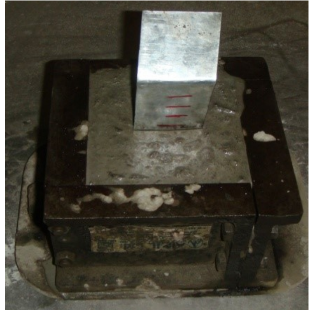
Figure 6. Steel plate induced in concrete cube
