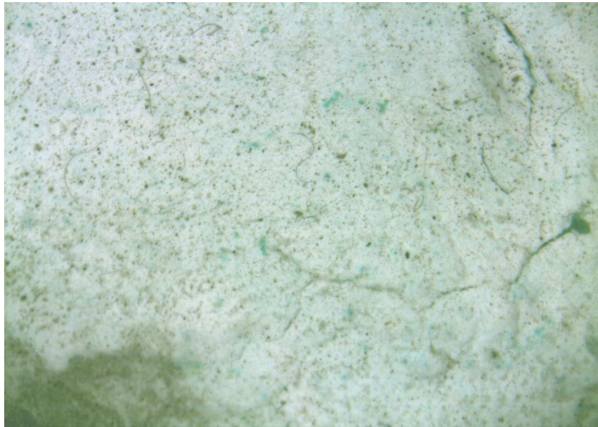
Figure 26. Cracks under Microscopic evaluation
