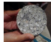
Figure 1. Section of microbial concrete
