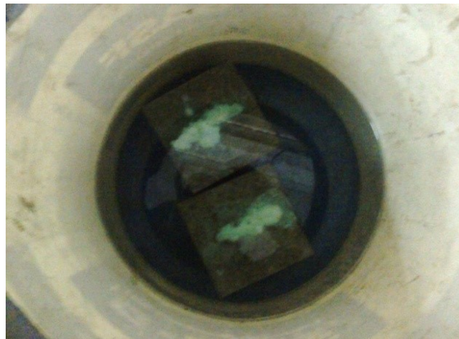
Figure 12. Cubes immersed in solution
