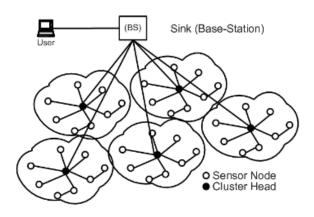
Figure 2. General Architecture of sensor network <sup>[6]</sup>
