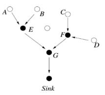
Figure 2 : Data Aggregation in WSNs
