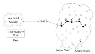
Figure 1: WSN Communication Architecture
