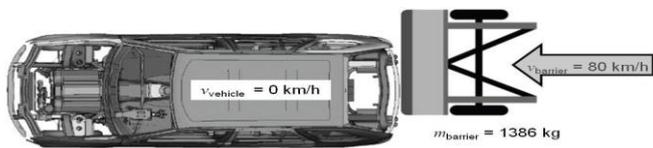
Figure 5: Rear impact test as defined in FMVSS 301.
