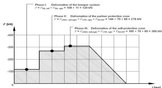
Figure 8: Crash phases for the rear impact.
