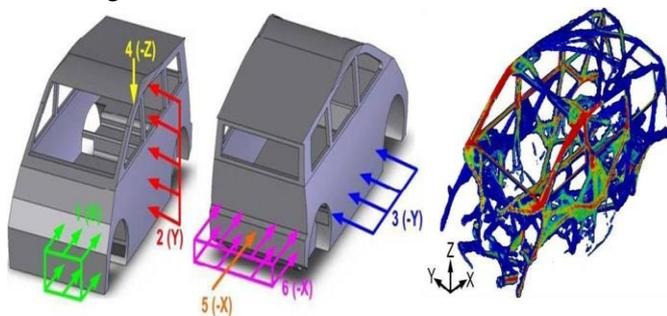
**Figure 1:** Equivalent static loads and optimization result [25].
