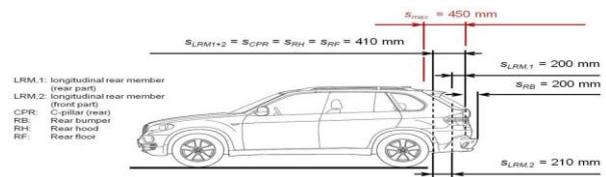
Figure 7: Free crash lengths for the rear impact.
