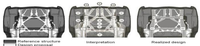
**Figure 11:** Optimized topology compared to the reference design and its interpretation.
