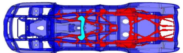
**Figure 13:** Topology optimization result (front, side and rear impacts).
