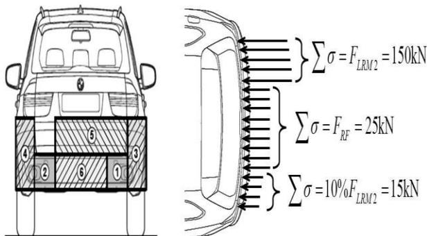
**Figure 9:** Load distribution for the rear impact (phase 2),
