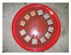
Figure 1. Setup for water sorptivity test
