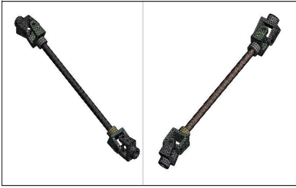
Fig.2. Meshed model for Propeller shaft assembly with 25 mm Mesh Size
