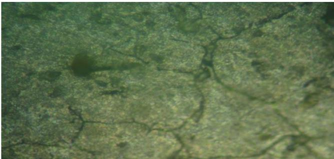
Plate 3: Micrograph of Al-5.6wt%Zn-2.5wt%Mg soaked for 90minutes and cooled in water
