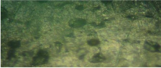
Plate 1: Micrograph of Al-5.6wt%Zn-2.5wt%Mg alloy (Control)
