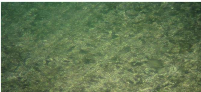
Plate 5: Micrograph of Al-5.6wt%Zn-2.5wt%Mg soaked for 30minutes and cooled in brine
