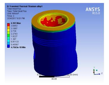
d) Titanium alloy total heat flux distribution
