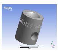
Figure 2.1 Model of the piston
