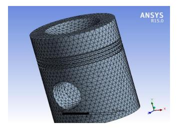
Figure 2.4 Meshing of Piston
