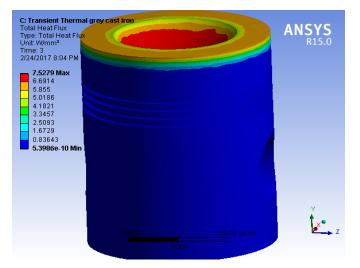
b) Grey cast iron total heat flux distribution
