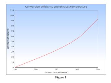
This high temperature required by the converter is a challenging aspect in automobile design. In the initial days, the catalytic converters were placed close to the engine to ensure faster heating. However, This location can cause two problems.
