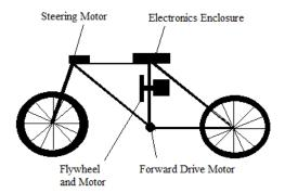
The flywheel design employs a flywheel which rotates about an axis parallel to the bicycle's frame. This design models the bicycle as a pendulum with a fixed pivot where the bicycle wheels meet the floor. As the bicycle begins to fall to one side, a motor mount to the bicycle exerts a torque on the flywheel, causing a reactionary torque on the bicycle, which restores the bicycle's balance.
