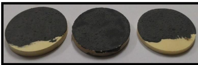
Figure 4.19 Coatings on alumina using sodium silicate binder
