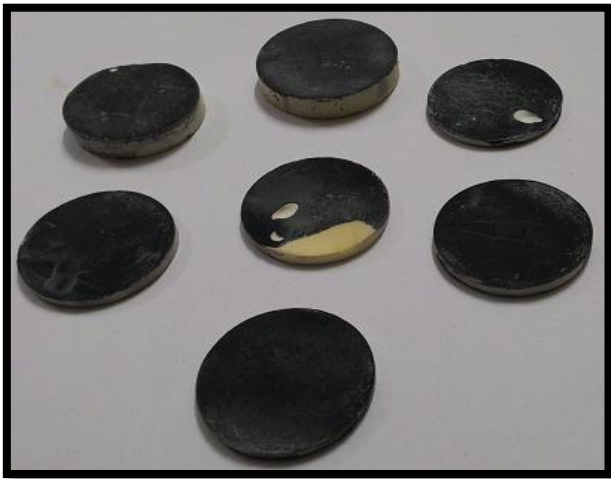
Figure 4.18 Coatings on alumina using aluminium phosphate binder.
