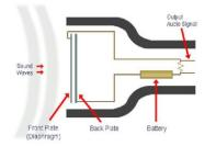
Figure 3. Cross Section of Microphone
