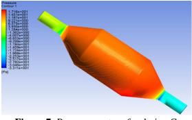
Figure 7: Pressure contour for design C
