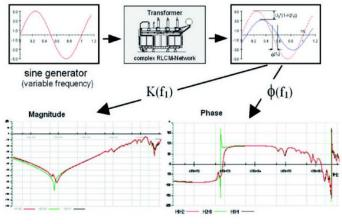
Figure 2: Basic principle of SFRA
