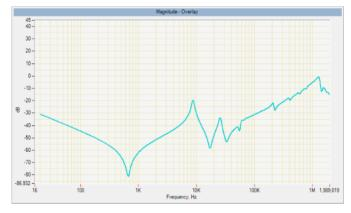
Figure 4 : HV winding between 1U and 1N at tap no:1, with LV open
