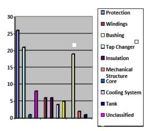
Figure 1: Failure in transformers
