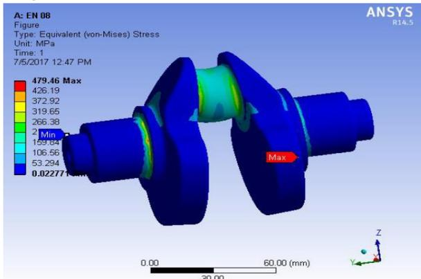
**Figure No : 8** Von Mises Stress Distribution (EN 8) of Crankshaft.
