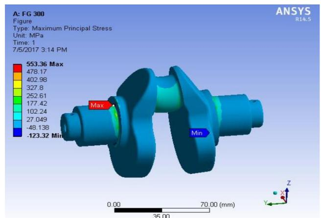
**Figure No : 7** Maximum Principal Stress (FG 300) of Crankshaft
