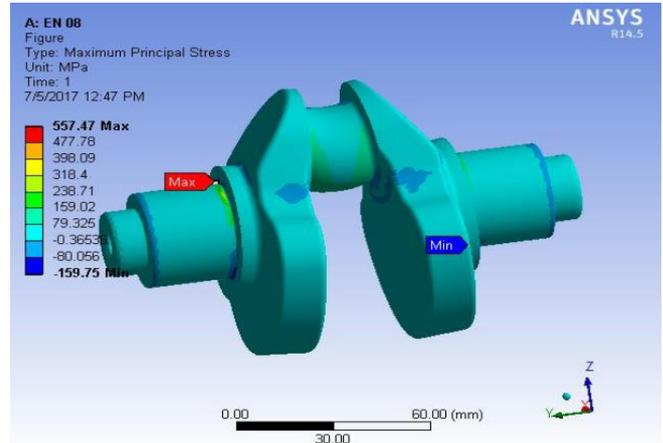
**Figure No : 10** Maximum Principal Stress (EN 8 material) of Crankshaft
