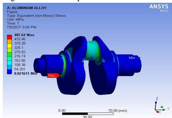
**Figure No : 14** Von Mises Stress (Aluminium Alloy) of Crankshaft.
