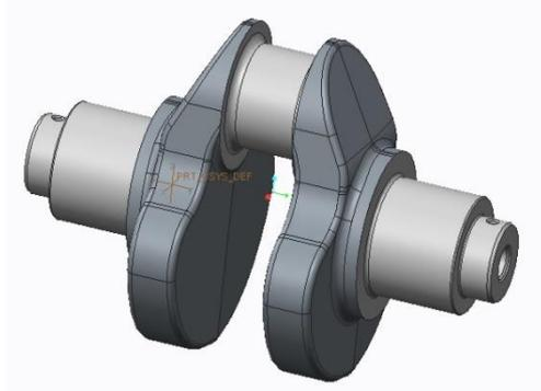
Figure No:- 1 Three Dimensional Modeling Original Crakshaft in Creo 2.0
