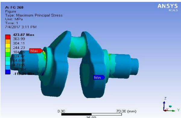
**Figure No: 4** Maximum Principal Stress (FG 260) of Crankshaft
