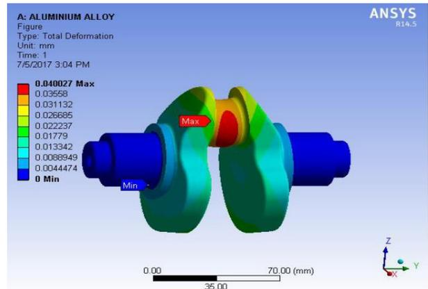
**Figure No : 15** Deformation of (Aluminium Alloy) Crankshaft
