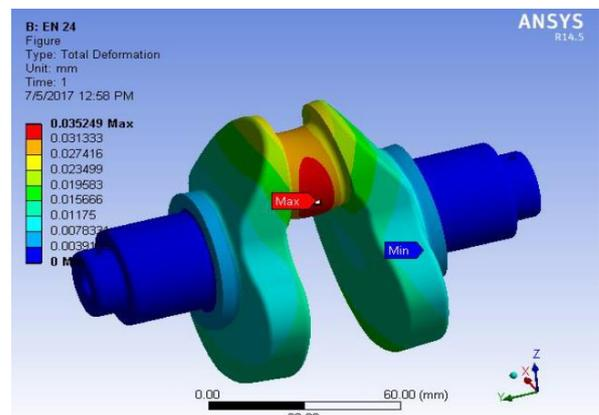
**Figure No : 12** Deformation of (EN 24) Crankshaft
