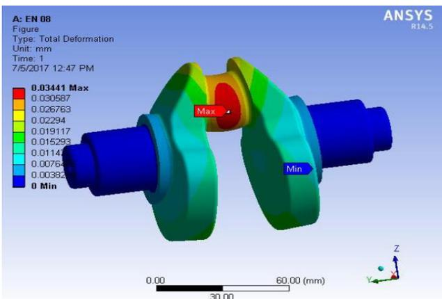
**Figure No : 9** Deformation of (EN 8 material) Crankshaft
