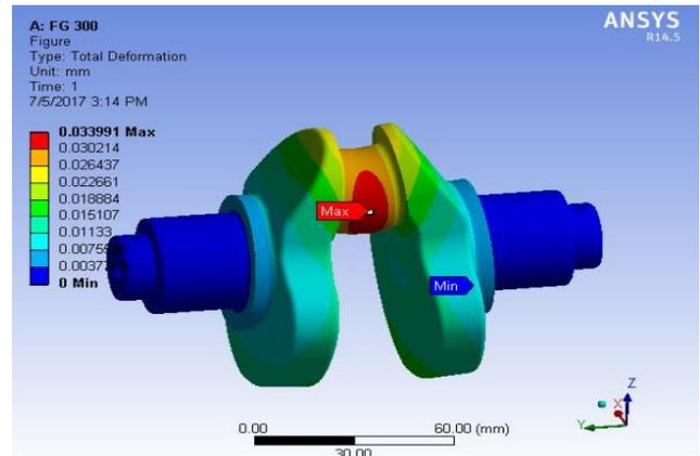
**Figure No :-6** Deformation of (FG 300) Crankshaft
