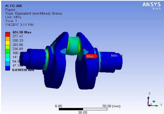
**Figure No : 2** Von Mises Stress Distribution (FG 260) of Crankshaft
