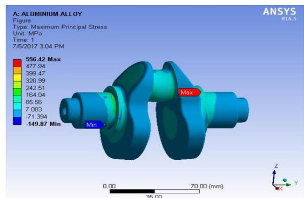
**Figure No : 16** Maximum Principal Stress (Aluminum Alloy) of Crankshaft
