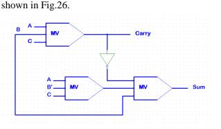
Figure.26. Proposed Full Adder Circuit Diagram with 3 MV gates
