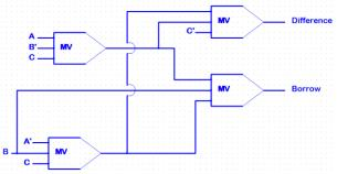
Figure.20. Full Subtractor Circuit Diagram with 4 MV gates[10]
