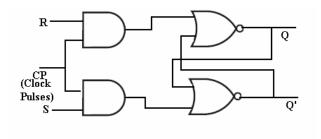
Figure 10. Conventional RS Flip Flop
