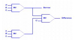
Figure.23. Full Subtractor Circuit Diagram with 3 MV gates
