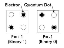
Figure.1. QCA cells showing how binary information is encoded in the two fully polarized diagonals of the cell[6].
