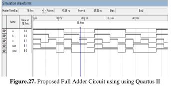
Figure.27. Proposed Full Adder Circuit using using Quartus II simulator.
