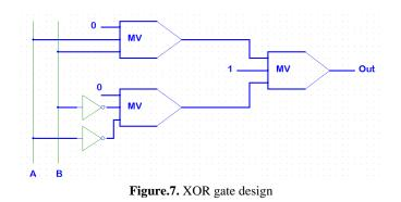
It is the designed use of majority gates and inverters. Formula (4) presents the equation of this gate. XOR = MV (MV (A, B,0), MV (A', B',0), 1) (4)
