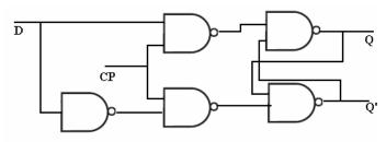
Figure 12. Conventional D Flip Flop
