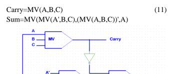
**Figure.25.** Proposed full Adder Circuit Diagram with 3 MV gates Also, the circuit diagram for the corresponding circuit is
