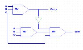
Figure.24. Full Adder Circuit Diagram with 3 MV gates[11]
