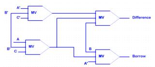
Figure.21.Full Subtractor Circuit Diagram with 4 MV gates[10]
