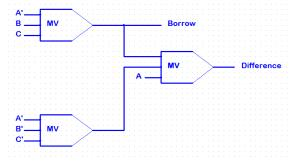
Figure.22.Full Subtractor Circuit Diagram with 3 MV gates
