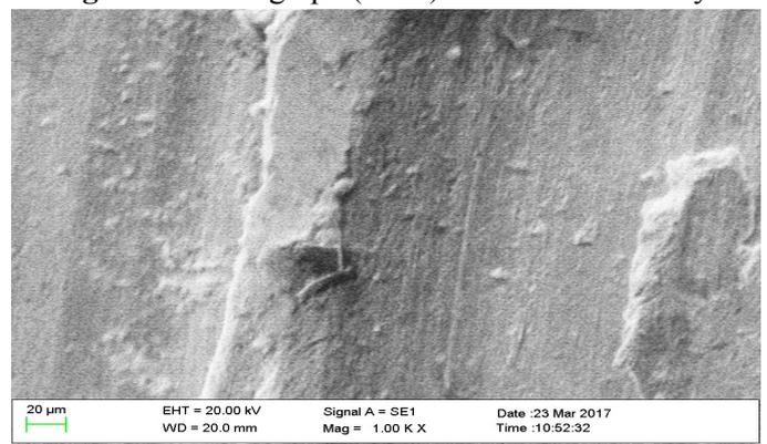
**Figure 9:** Micrograph (SEM) of Cu-3wt%Si-1wt%Sn alloy
