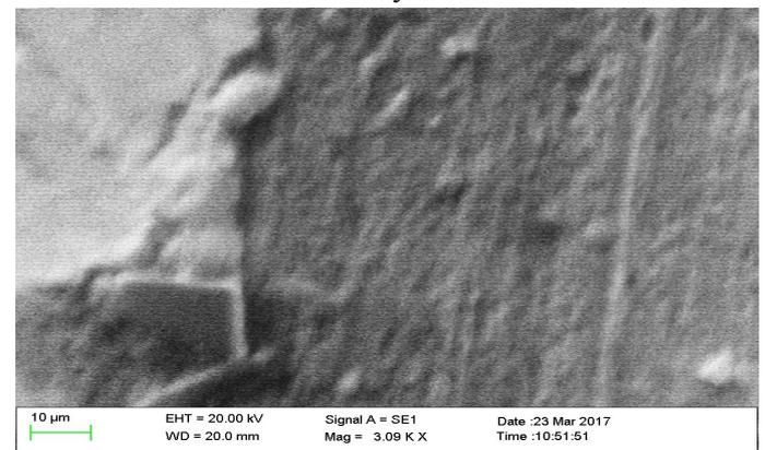
**Figure 10:** Micrograph (SEM) of Cu-3wt%Si-1.5wt%Sn alloy
