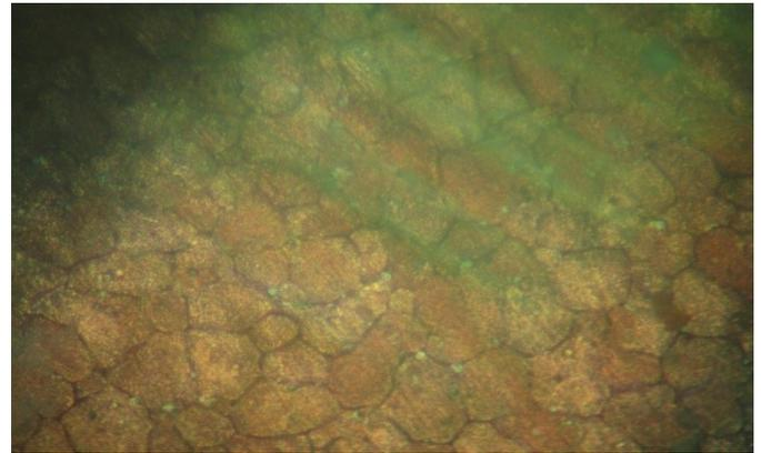
**Figure 7.** Micrograph of Cu-3wt%Si-1wt%Sn alloy
