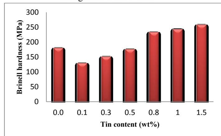
**Figure 3:** Effect of tin content on the hardness of silicon bronze
