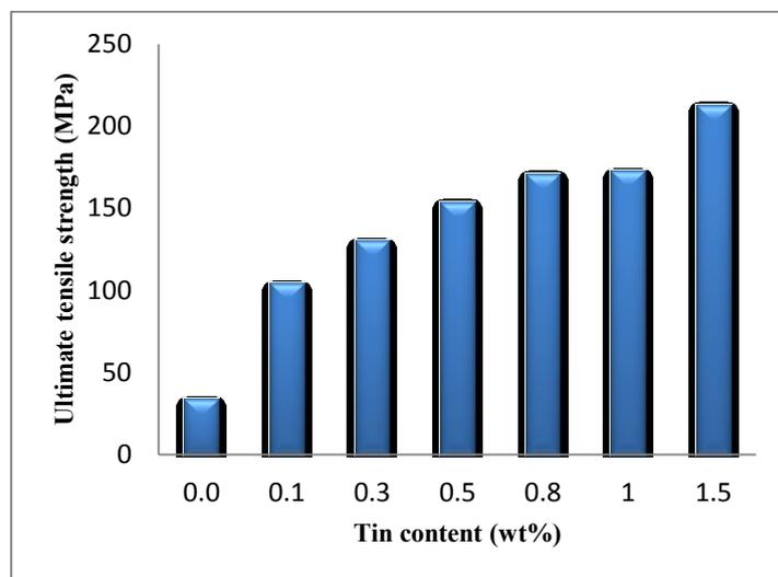
**Figure 2:** Effect of tin content on the ultimate tensile strength of silicon bronze
