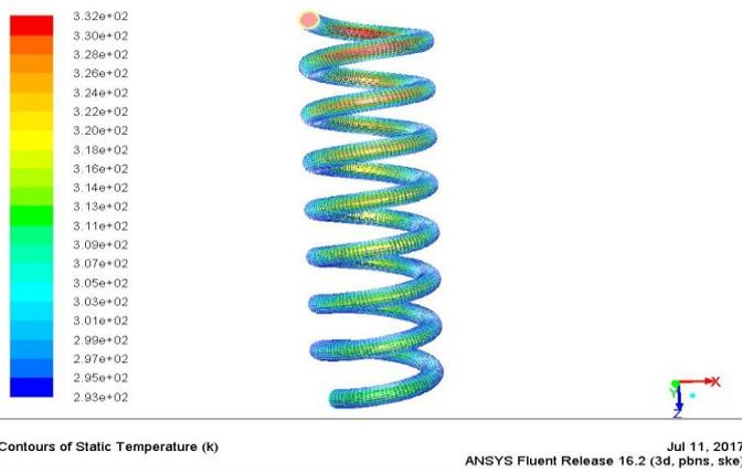
**Figure 5:** Temperature variation for 8 mm coil diameter for mass flow rate of 0.02 Kg/s.
