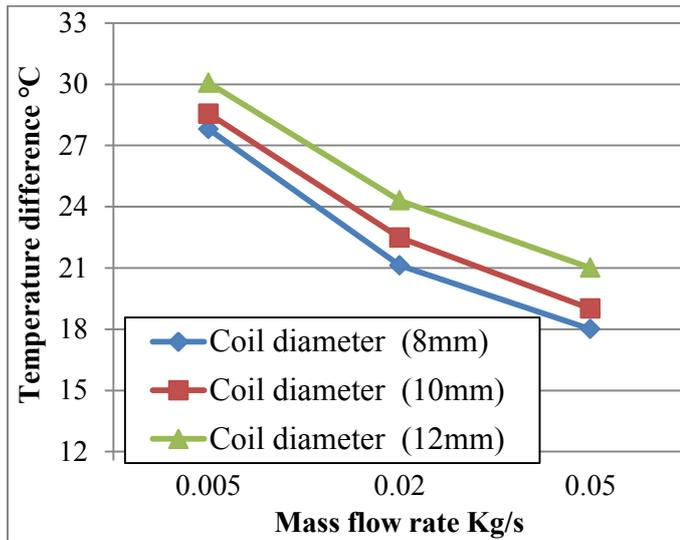
**Figure 9:** Variation in temperature drop with mass flow rate at different diameter.
