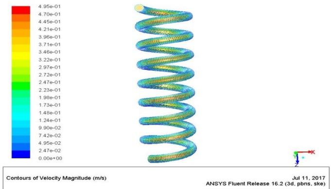
**Figure 7:** Velocity variation of fluid in 8 mm coil diameter for mass flow rates of 0.02Kg/s.
