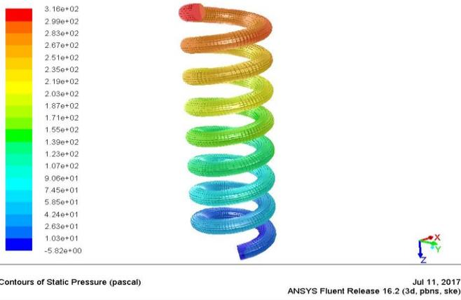
**Figure 4:** Pressure variation for 10mm coil diameter for mass flow rate of 0.02 Kg/s.
