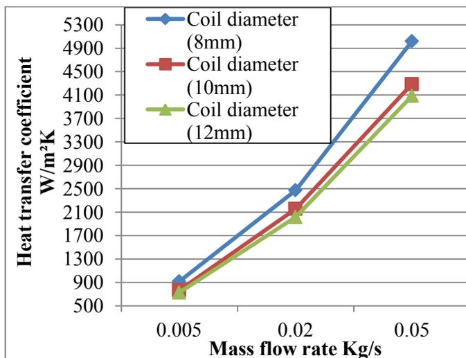
**Figure 10:** Variation in heat transfer coefficient with mass flow rate at different diameter of coil.
