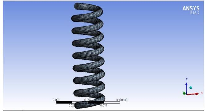
Figure 2: 3D view of mesh of helical coil heat exchanger
