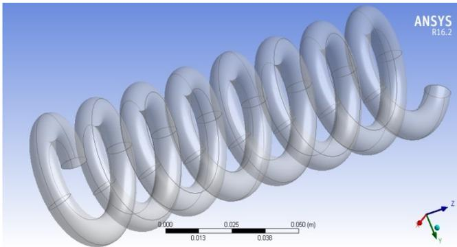
Figure 1: 3D view of helical coil heat exchanger
