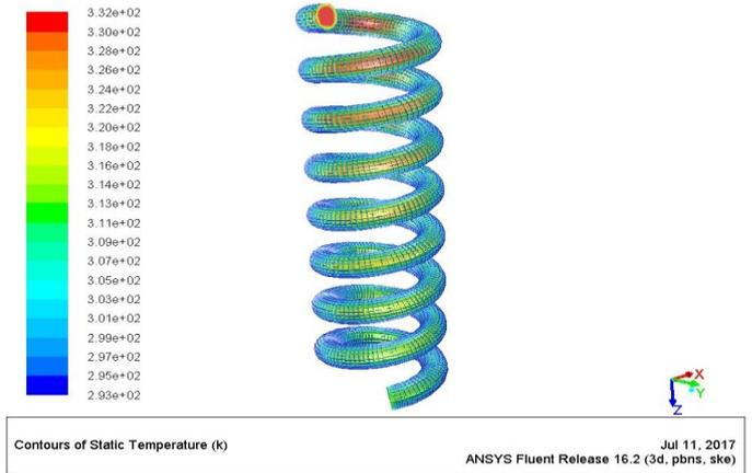
**Figure 6:** Temperature variation for 10mm coil diameter for mass flow rate of 0.02 Kg/s.
