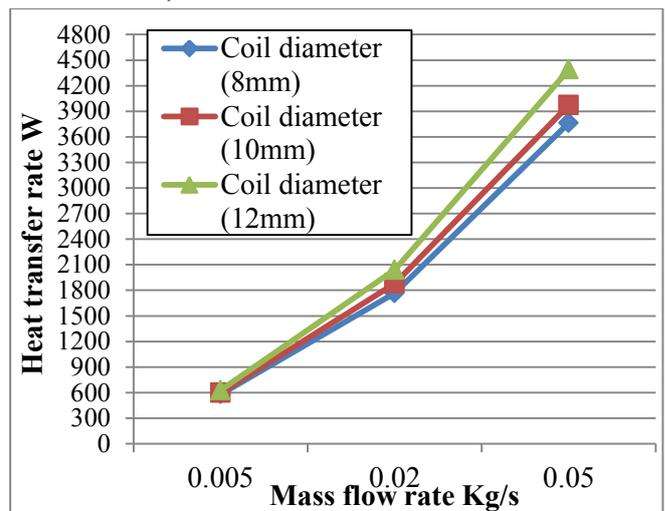
**Figure 12:** Variation in heat transfer rate with mass flow rate at different coil diameter.
