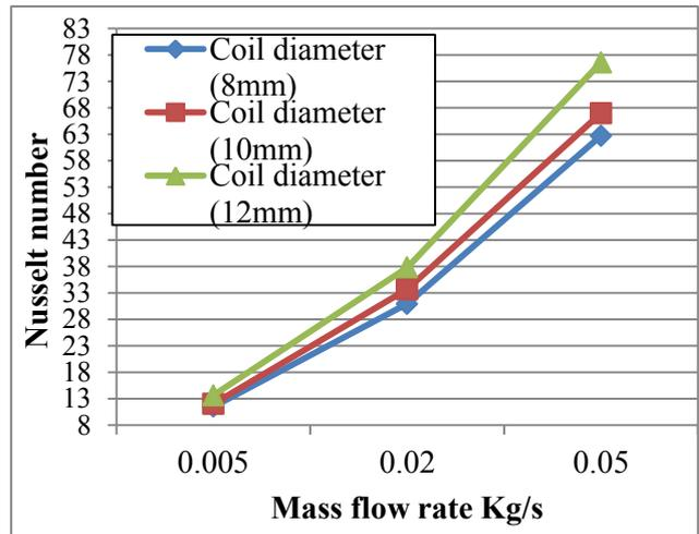
**Figure 11:** Variation in Nusselt number with mass flow rate for different coil diameter.
