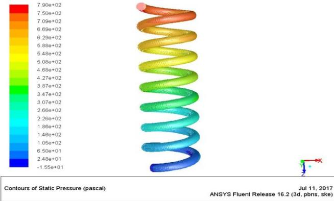
**Figure 3:** Pressure variation for 8mm coil diameter for mass flow rate of 0.02 Kg/s.
