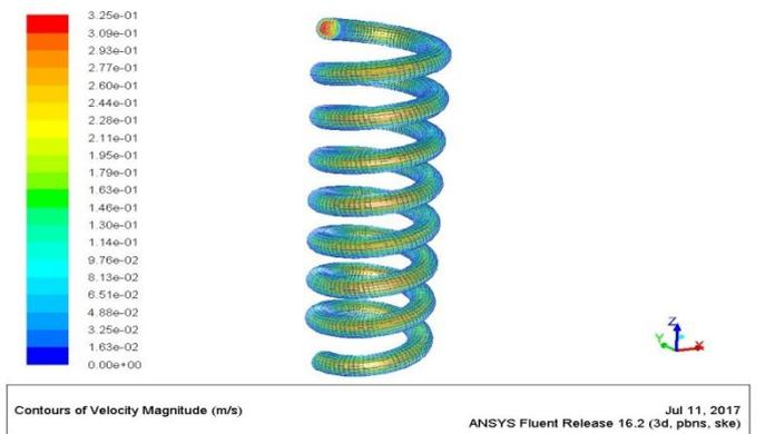
**Figure 6:** Velocity variation of fluid in 10 mm coil diameter for mass flow rates of 0.02Kg/s.
