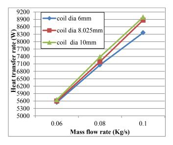
Figure 3: Variation in heat transfer rate with diameter
