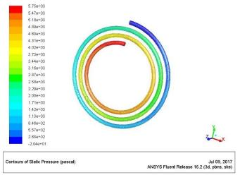
Figure 8: Variation in pressure for 10mm coil diameter at 0.06 kg/sec mass flow rate
