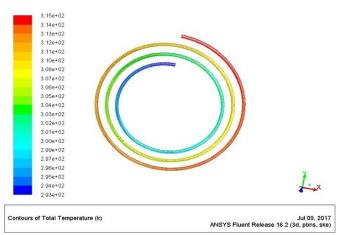
**Figure 6:** Variation in temperature for 6mm coil diameter at mass flow rate of 0.06 Kg/s.
