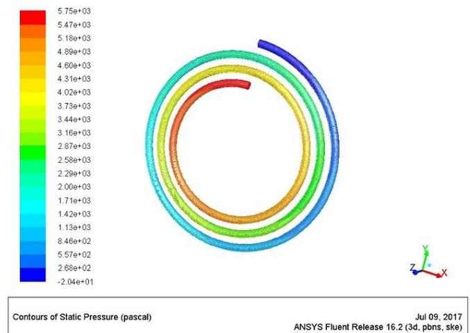
**Figure 8:** Variation in pressure for 10mm coil diameter at 0.06 kg/sec mass flow rate
