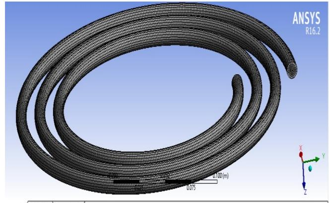
Figure 2 :3 Dimensional view of mesh of spiral coil heat exchanger
