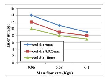
**Figure 4:** Variation in Euler No. for 6mm, 8.025mm & 10mm coil diameter of spiral coil heat exchanger.
