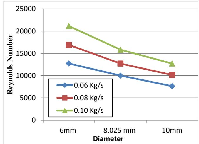
**Figure 5:** Variation of Reynolds No. on 6mm, 8.025mm & 10mm diameter
