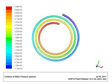
Figure 7: Variation in pressure for coil diameter 8.025 mm at 0.06 kg/sec mass flow rate
