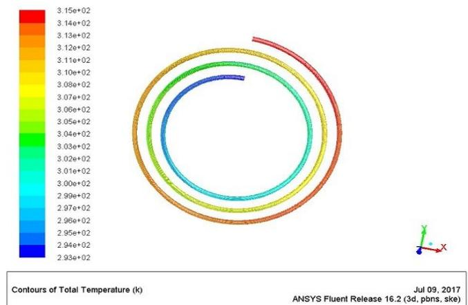
**Figure 6:** Variation in temperature for 6mm coil diameter at mass flow rate of 0.06 Kg/s.
