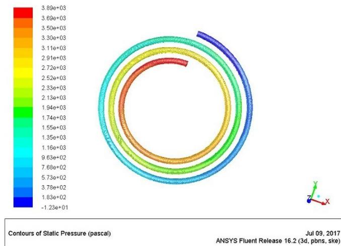
**Figure 7:** Variation in pressure for coil diameter 8.025 mm at 0.06 kg/sec mass flow rate
