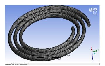
Figure 2 shows the mesh of spiral coil heat exchanger of 6mm tube diameter.
