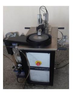
Figure 2. Pin on disc wear test apparatus
