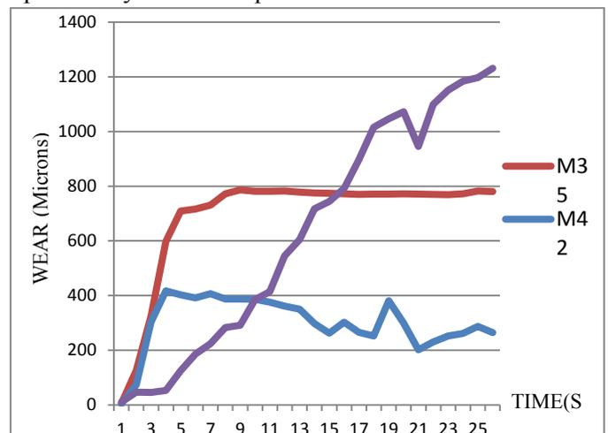
**Figure 3.** Graph of comparison of wear of selected materials for optimum heat treatment cycle
