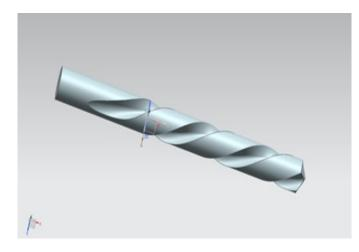
Figure 1. Ground Flute Twist Drill Tool
