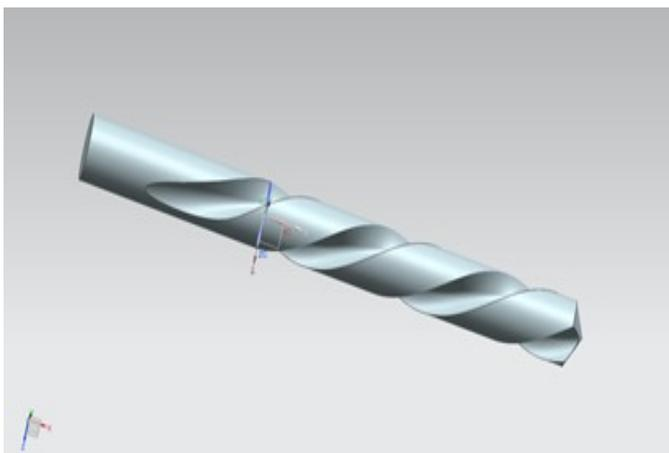
**Figure 1.** Ground Flute Twist Drill Tool
