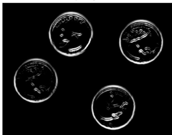
**Figure 42.** Fuzzy logic based Edge Detector Results
