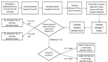
Figure 1: Flowchart of Selective Algorithm
