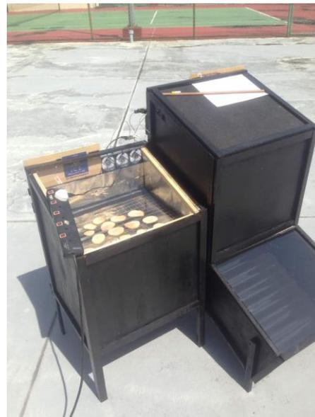
**Figure 2:** The front of direct dryer (left) and indirect dryer (right)
