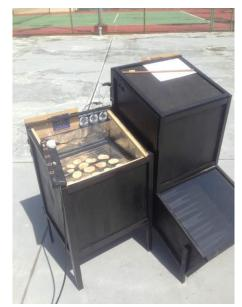
Figure 2: The front of direct dryer (left) and indirect dryer (right)
