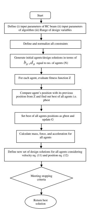
Figure2: Flow chart for RC beam optimal design using PSOGSA
