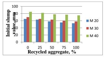
Figure 3 : Initial slump value for RAC mixes of different grades
