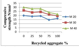
Figure 4: Compressive strength of concrete at 7 days
