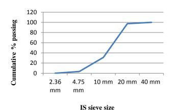
Figure 1: Gradation curve for coarse aggregates- NA
