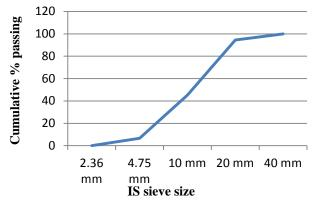
Figure 2: Gradation curve for coarse aggregates- RA
