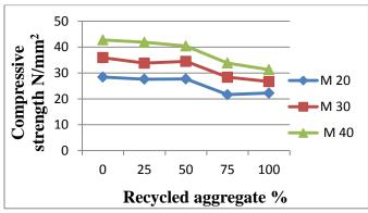
Figure 5: Compressive strength of concrete at 28 days
