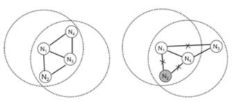
Figure 2. an illustration, where a failed node is shaded and a link with a cross mean that the link is down.
