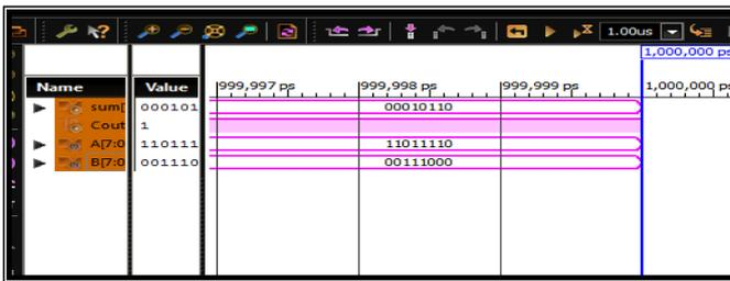
Figure 5 : Ripple Carry Adder Output
