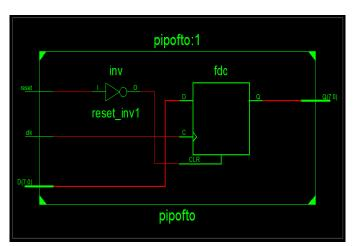
Figure 3. 8 bit PIPO RTL schematic view in Xilinx
