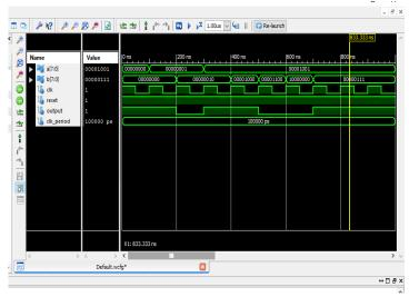
Figure 2. Test-bench simulation of 8 bit comparator created in Xilinx
