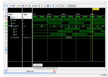
Figure 6. Test-bench simulation of 3 bit SIPO register created in Xilinx
