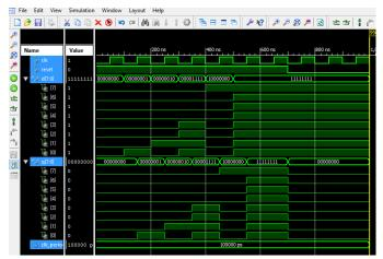
Figure 4. Test-bench simulation of 8 bit PIPO register created in Xilinx
