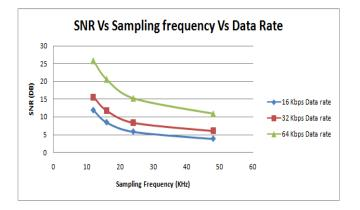
The SNR calculated at different data rates at different frequencies. Here if we increase the data rate of the CVSD system the signal to noise ratio is increases and if we increase the sampling frequency of the input signal then comparison of the comparator is decreases so signal quality at output of decoder is decreases so SNR is decreases.
