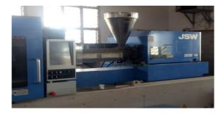
Figure 2. Injection Moulding Machine: JSW 180H
