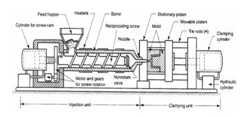
Figure.1 Injection Moulding Machine
