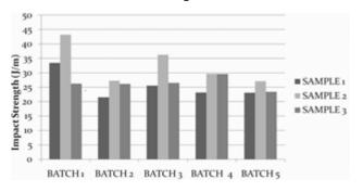
**Table 3**. impact strength of PP composites at different filler loadings.
