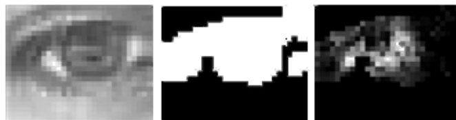
Figure 4: Left to right: A blurred eye image; the areas considered dark enough to be pupil candidates; our estimates of center probability in the regions that were dark (white=highest probability). Note the spurious peak on the left.
